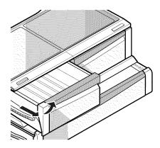
**3.** To install, slightly tilt up the front, insert the drawer into the frame and push it back into place.
